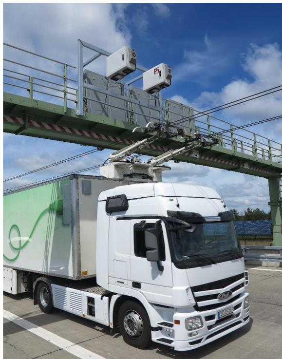
Figure 1: PantoSystem installed on first eHighway test track in Germany
