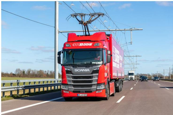
Figure 2: eHighway trucks with new pantograph design on German highway roads
