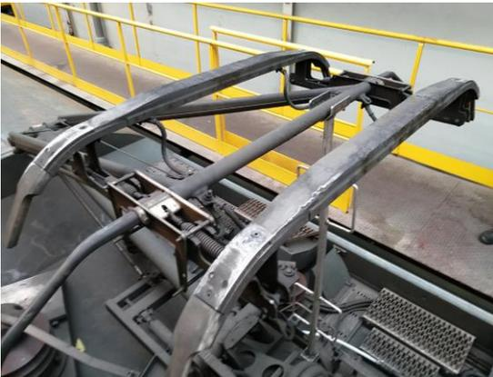
Figure 1: The damaged pantograph
