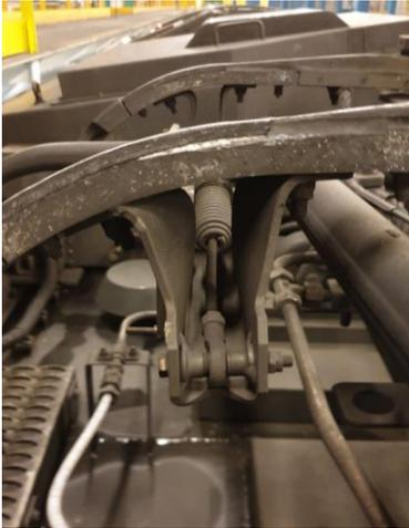
Figure 3: Broken spring box
