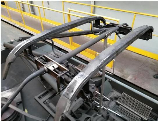
Figure 1: The damaged pantograph
