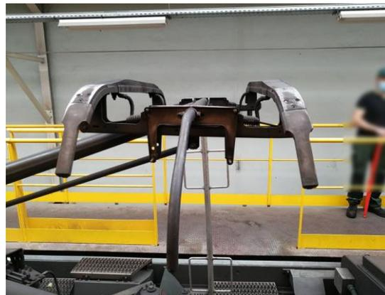
Figure 2: Carbon strip shows clear pitch
