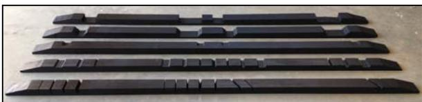
**Figure 12: Wooden carbon strips with simulated defects**
