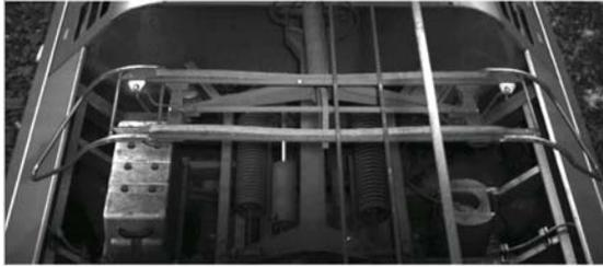
**Figure 4: Operator viewable photograph of the pantograph**
